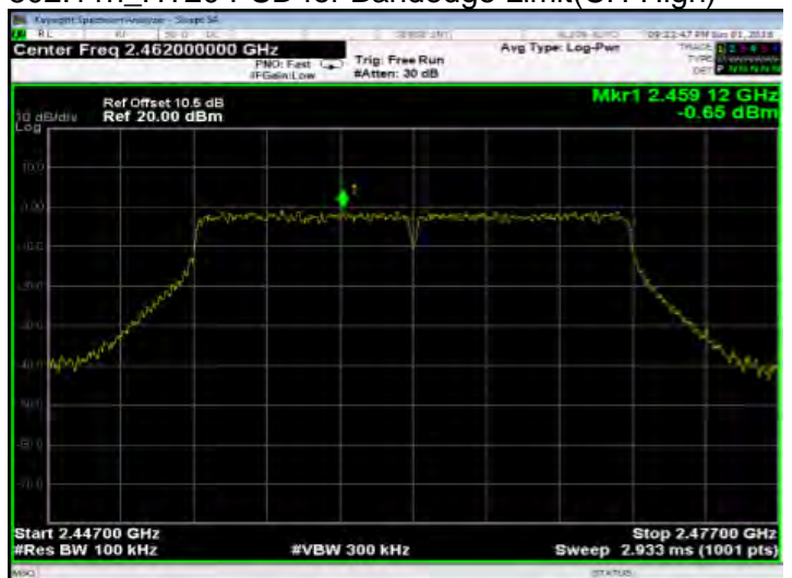
802.11n_HT20 PSD for Bandedge Limit(CH-High)
