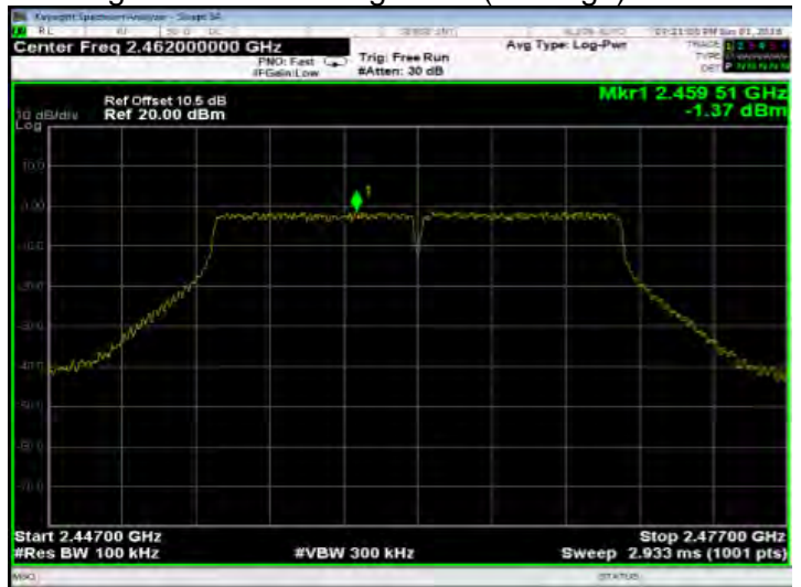
802.11n_HT20 PSD for Bandedge Limit(CH-Low)
