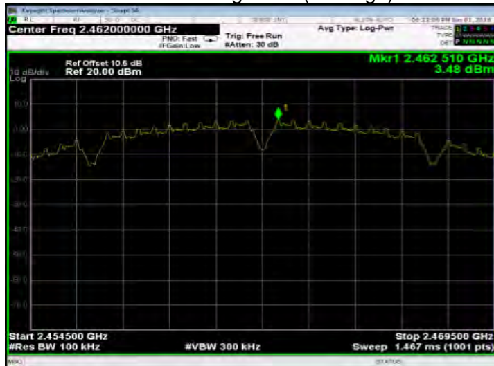
802.11g PSD for Bandedge Limit(CH-Low)
