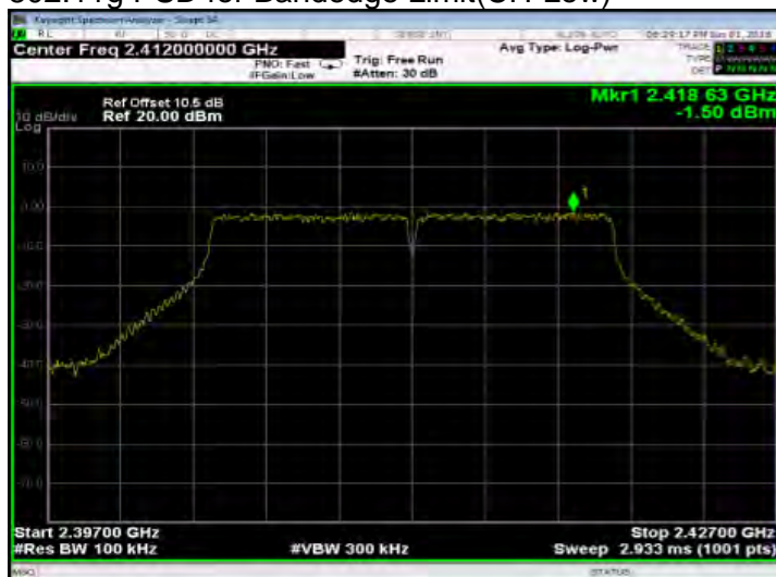
802.11g PSD for Bandedge Limit(CH-Low)
