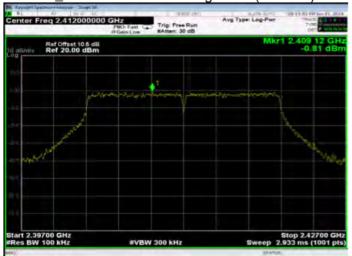
802.11n_HT20 PSD for Bandedge Limit(CH-High)
