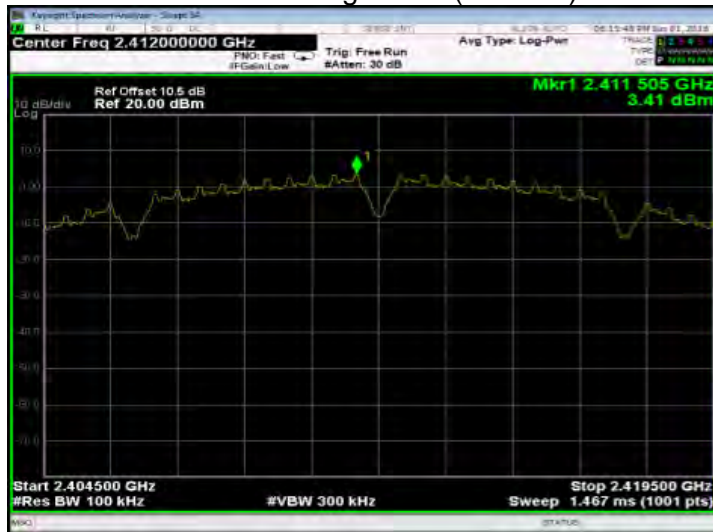
802.11b PSD for Bandedge Limit(CH-High)
