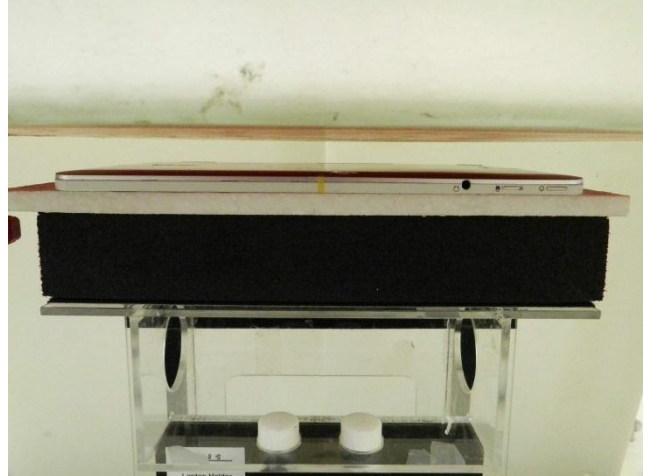
Bottom Face with Phantom 1.5 cm Gap
