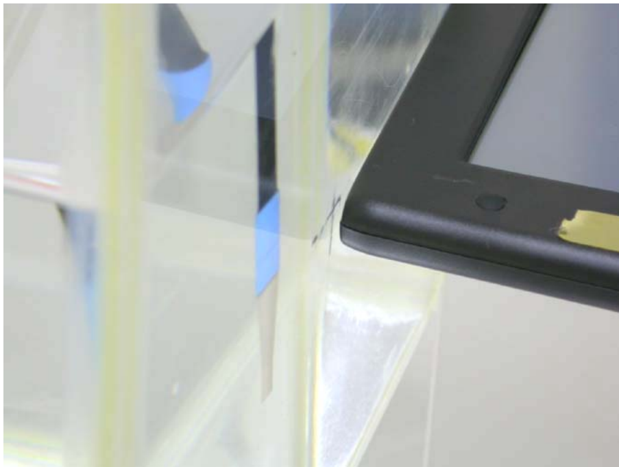
Figure: 11 EUT right to phantom, 0 mm separation- Zoom In
