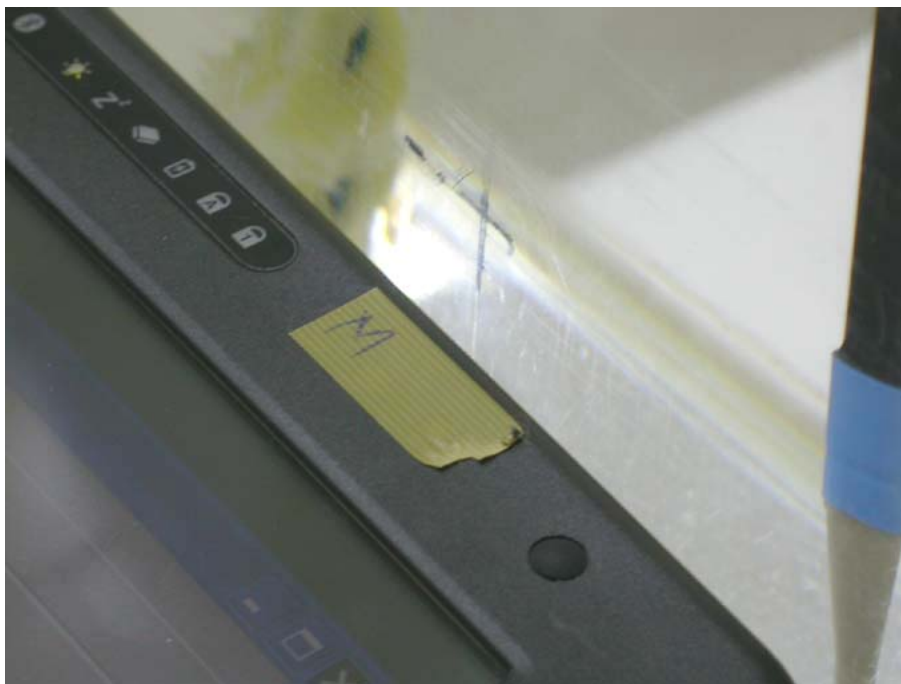
Figure: 3 EUT top to phantom, 0 mm separation– Zoom In
