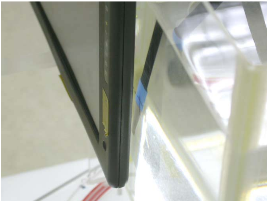
Figure: 7 EUT rear to phantom, 0 mm separation– Zoom In
