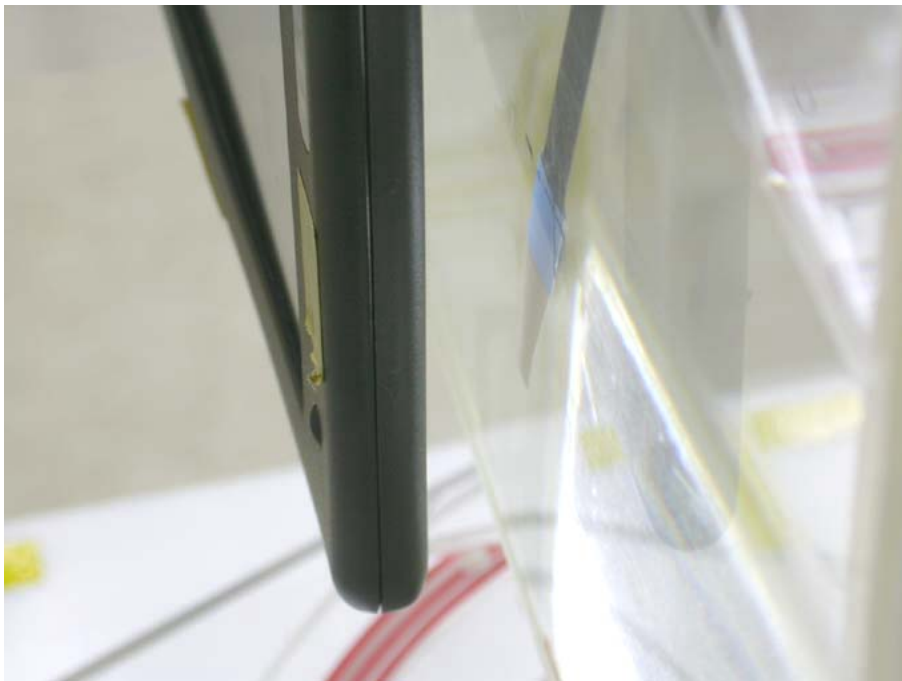
Figure: 9 EUT rear to phantom, 15 mm separation– Zoom In
