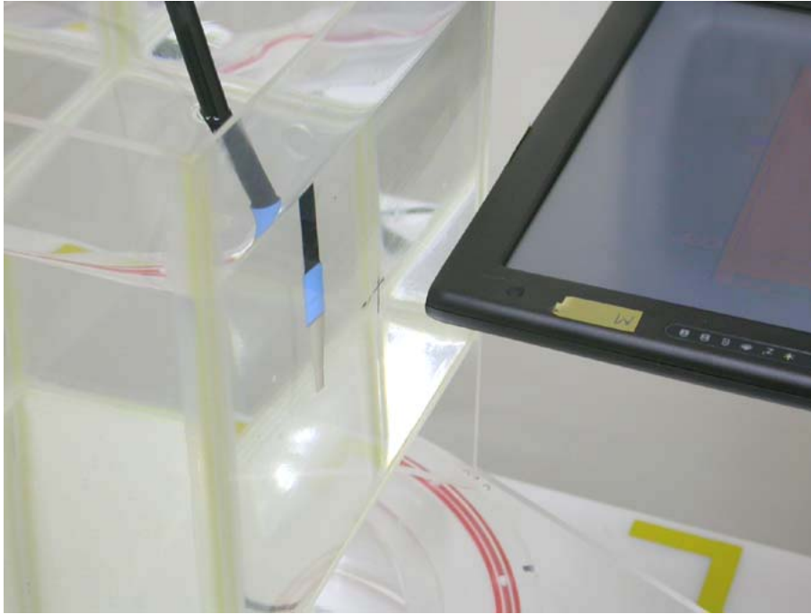
SAR Measurement Test Setup Figure: 12 EUT right to phantom, 15 mm separation
