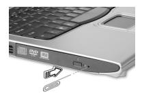
When the power is off, you can eject the drive tray by using the emergency eject hole.
