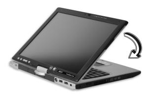
4 Remove the EMR stylus from the pen slot to begin pen-based input.
