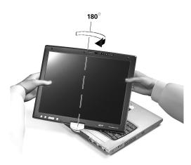
3 With the screen facing away from the keyboard, close the display cover and slide the lock lever to properly secure the screen.
