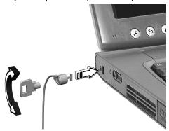
Wrap the computer security lock cable around an immovable object such as a table or handle of a locked drawer. Insert the lock into the notch and turn the key to secure the lock. Some keyless models are also available.
