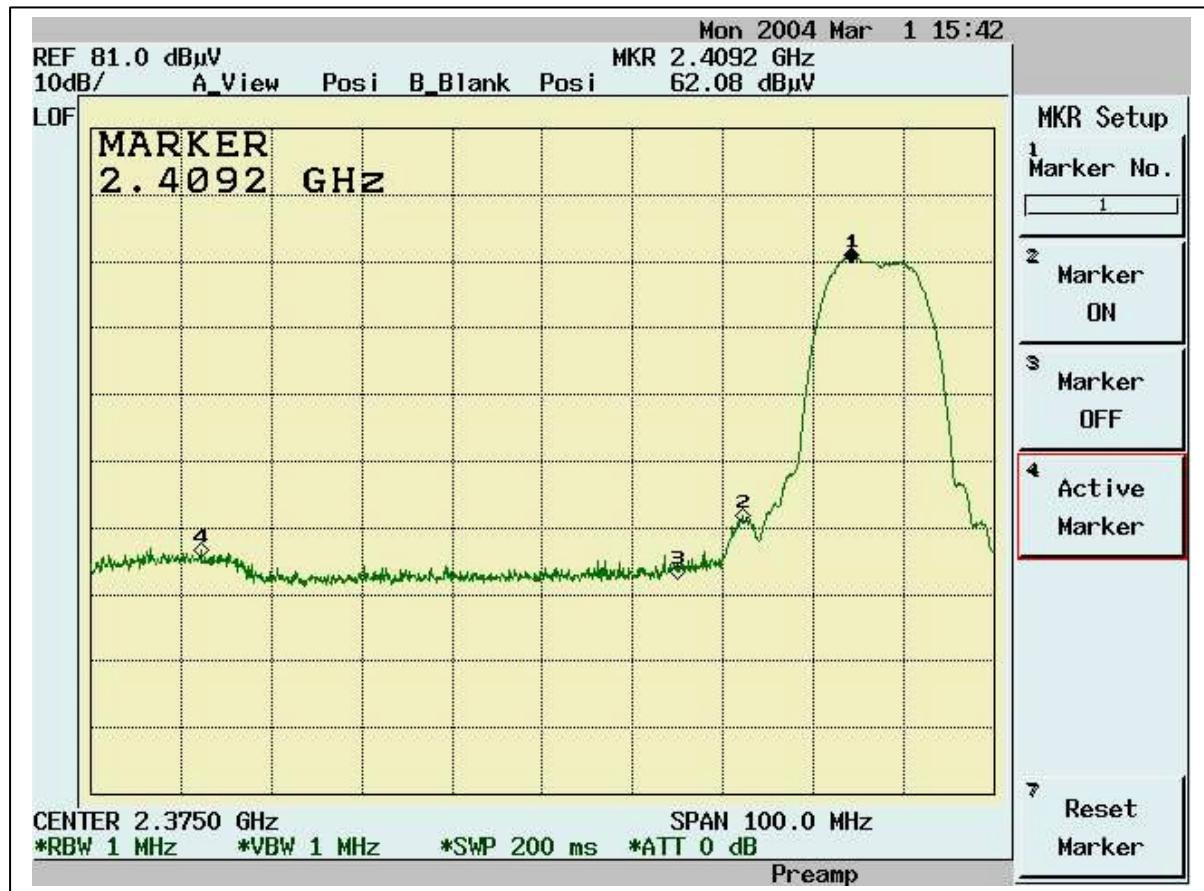
**Band Edge measurement for radiated emission in Restricted Band(Radiated)****Average Mode (Channel 1)**
