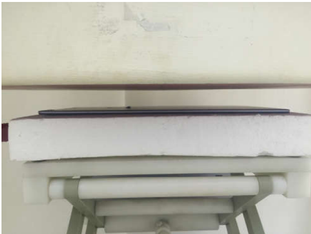
Back of Display Screen, Test Separation 25 mm
