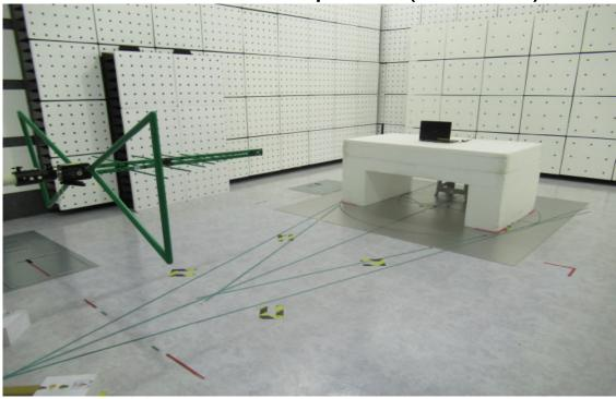
Radiated Emission Set up Photos (Above 1GHz)
