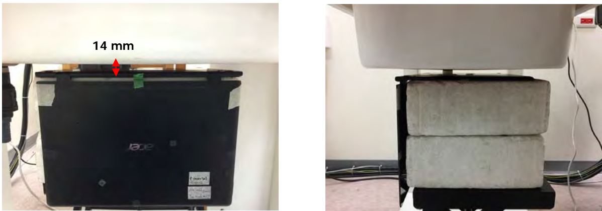
Fig.4 EUT Bottom side to flat phantom
