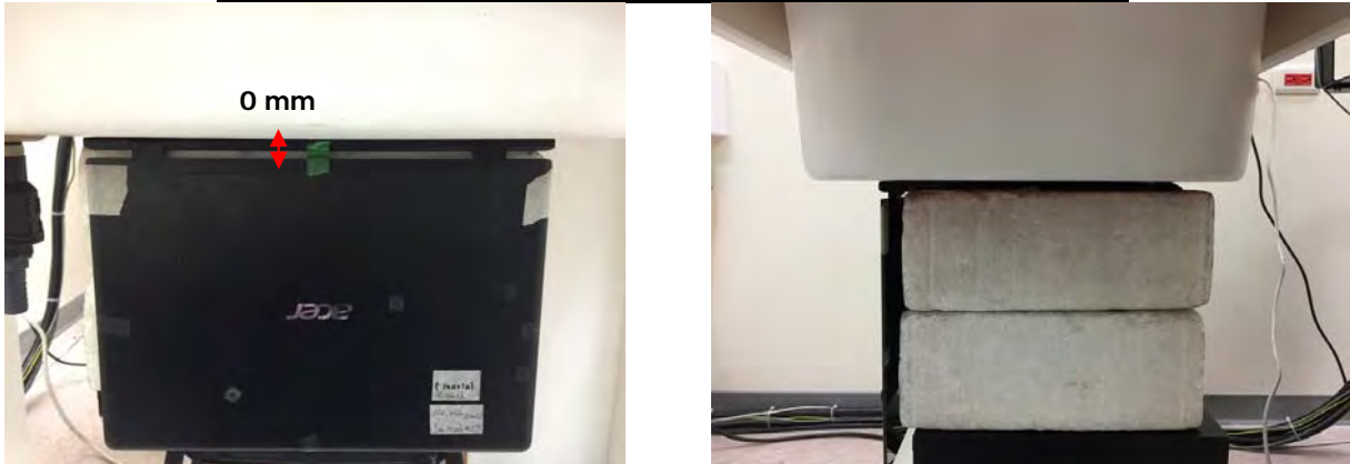
Fig.3 EUT Bottom side to flat phantom
