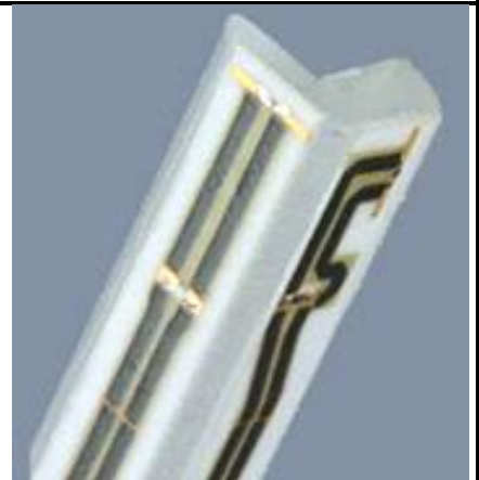
Fig 5.2 Photo of E-field Probe
