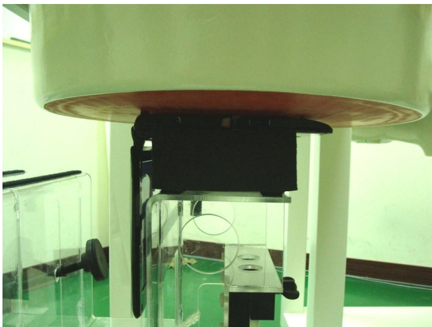
Side View - Bottom of DUT with Phantom 0cm Gap (KAV60 with GSM/WCDMA Antenna)
