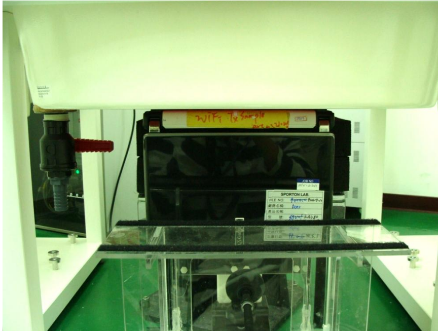
Rear View - Bottom of DUT with Phantom 0cm Gap (KAV80 with CDMA2000 Antenna)
