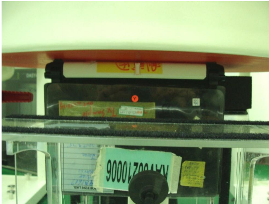
Rear View - Bottom of DUT with Phantom 0cm Gap (KAV60 with GSM/WCDMA Antenna)
