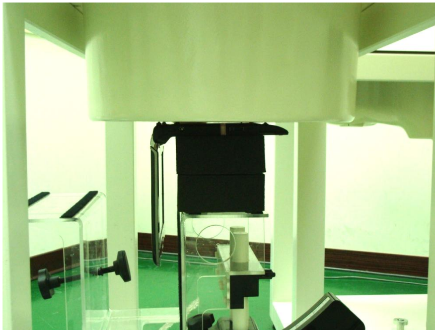
Side View - Bottom of DUT with Phantom 0cm Gap (KAV80 with CDMA2000 Antenna)
