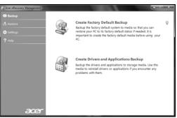
2 To create recovery discs for the hard drive's entire original contents, including Windows and all factory-loaded software and drivers, click Create Factory Default Disc.
