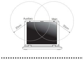
**Note:** The wireless Mini PCI adapter implements a transmission diversity function. The function does not emit radio frequencies simultaneously from both antennas. One of the antennas is selected automatically or manually (by users) to ensure good quality radiocommunication.
