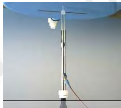
Photograph of the dipole Antenna
