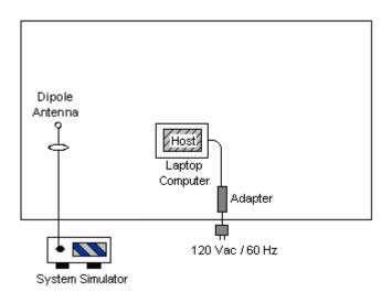
Remark: The EUT was 3G Module which was installed in the host laptop computer (Brand Name: Acer, Gateway, PackardBell / Model Name: ZH8, ZH7 / Marketing Name: Aspire one, AS1810T, AS1410, AS1810TZ; EC14 series, EC18 series; dot m/u; dor mr/u).
