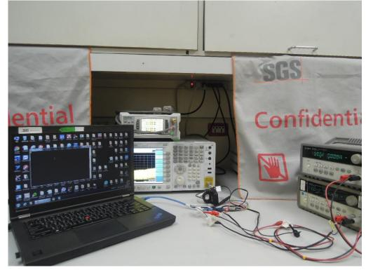
**BLE 2M Conducted Setup Photo (Measurement at Antenna Port)**
