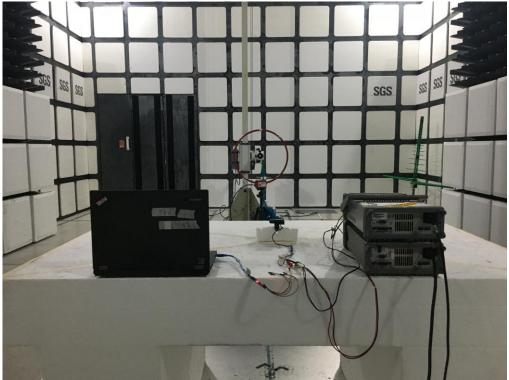
Radiated Emission Set up Photos (Below 1GHz)
