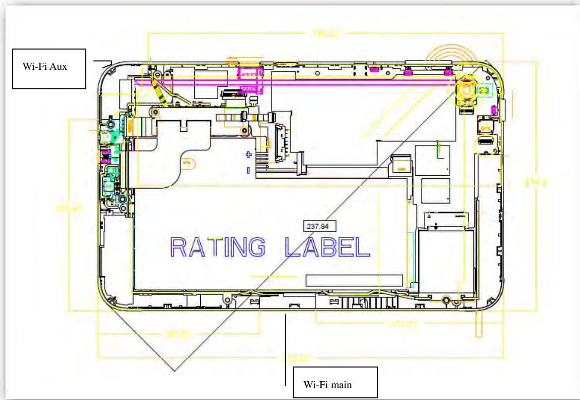
Fig.9 Antenna position of EUT
