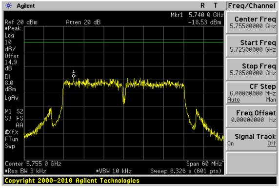
**Power Spectral Density Test Plot (CH-High)**
