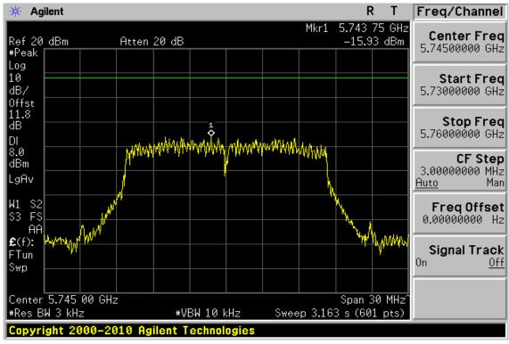
**Power Spectral Density Test Plot (CH-Mid)**
