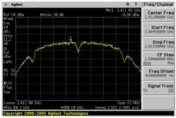
**Power Spectral Density Test Plot (CH-Mid)**
