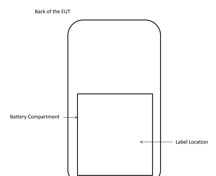
Label locates in the battery compartment and is visible to the users as they install the SIM card.
