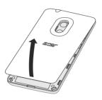
Insert your fingernail into the notch located at the bottom of the phone and remove the cover as illustrated. Ensure the microSD card and SIMs are inserted all the way
