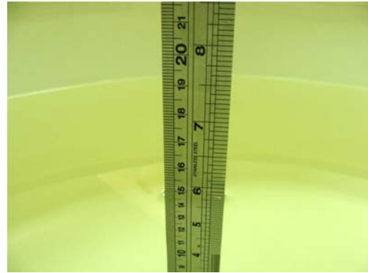
Fig 6.2 Photo of Liquid Height for Body SAR
