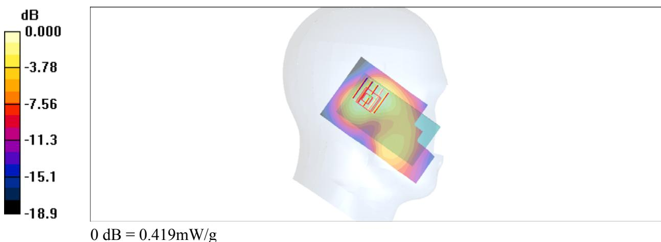
**#05 GSM1900\_DTM5\_Right Cheek\_Ch661****DUT: 242016**
