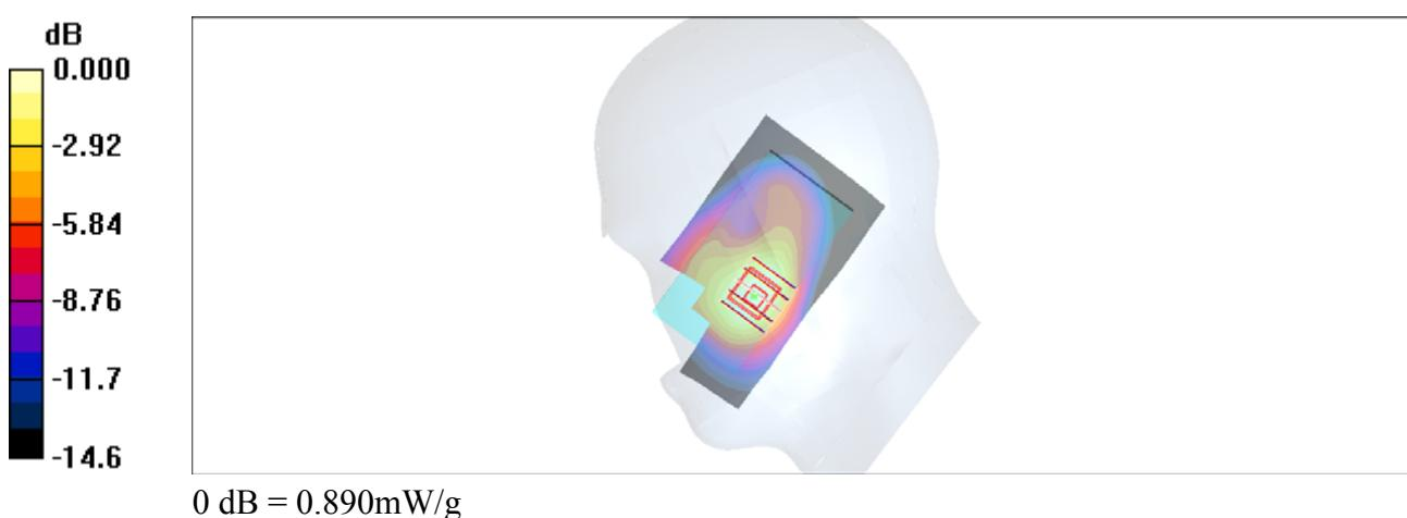
**#01 GSM1900\_DTM5\_Right Cheek\_Ch512\_2D****DUT: 242016**
