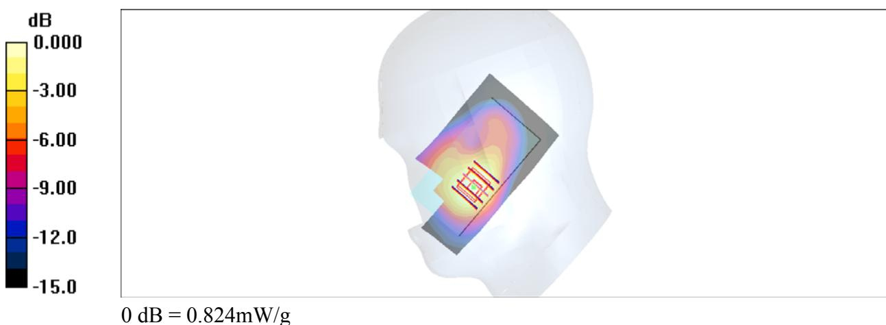
**#06 GSM1900\_DTM5\_Right Cheek\_Ch810****DUT: 242016**
