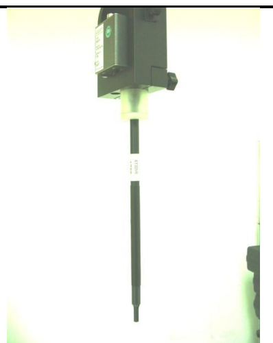
Fig 5.2 Photo of ET3DV6/ET3DV6R
