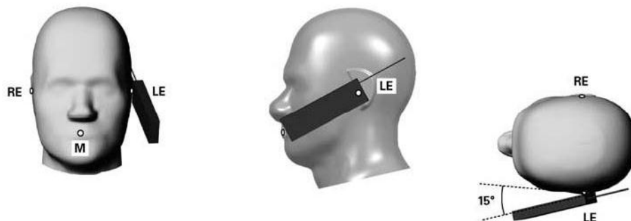
Fig 9.3 Illustration for Tilted Position
