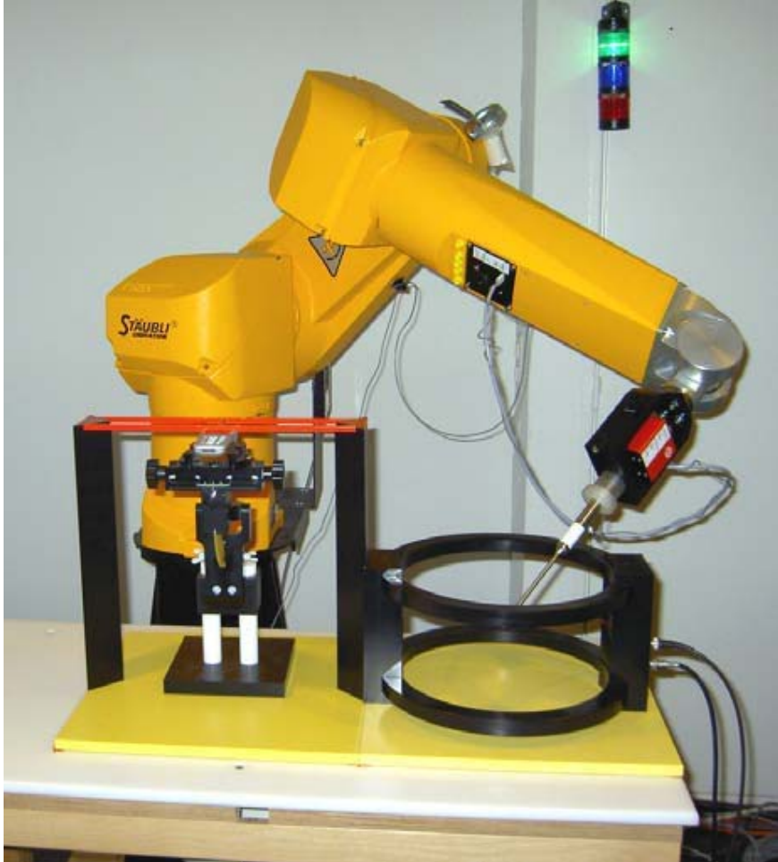
Figure 4.1: T-Coil setup with HAC Test Arch and AMCC
