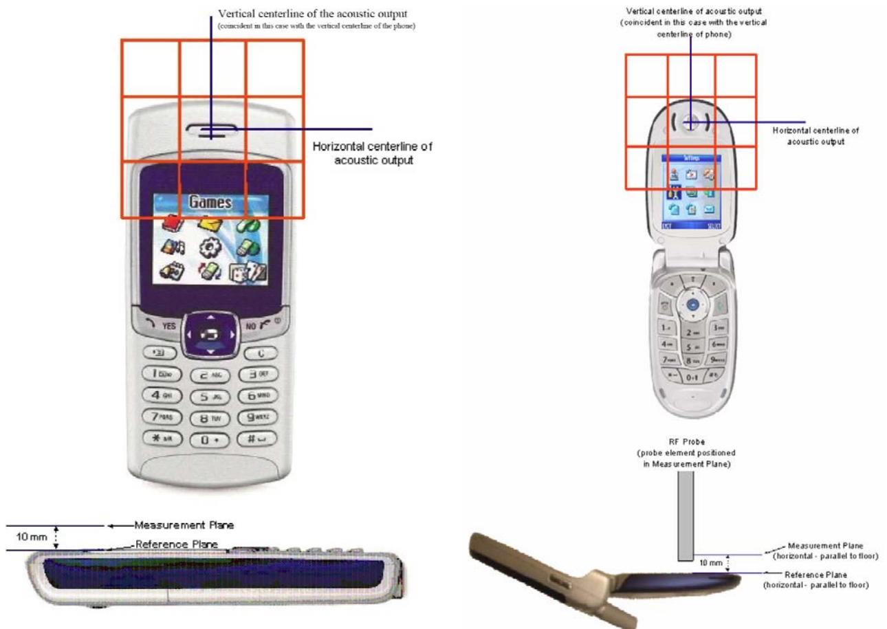
Figure 5.1: A typical DUT reference and plane for HAC measurements
