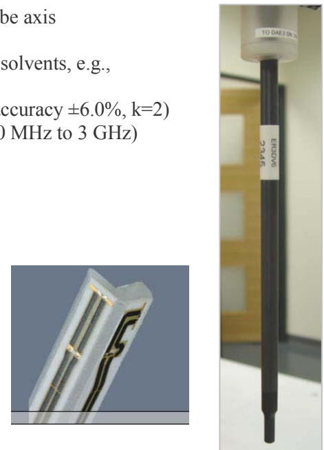
Figure 4 and 5: ER3DV6 E-Field Probe
