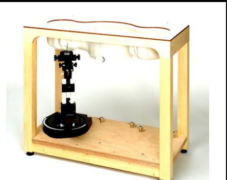
Fig 5.9 Photo of SAM Phantom
