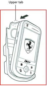
6 Adjust the car pedestal for the best viewing angle.
