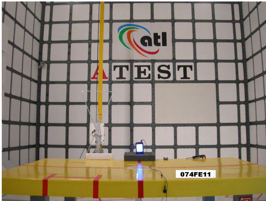
Figure 9. Front View of the Test Configuration (Car Charge)
