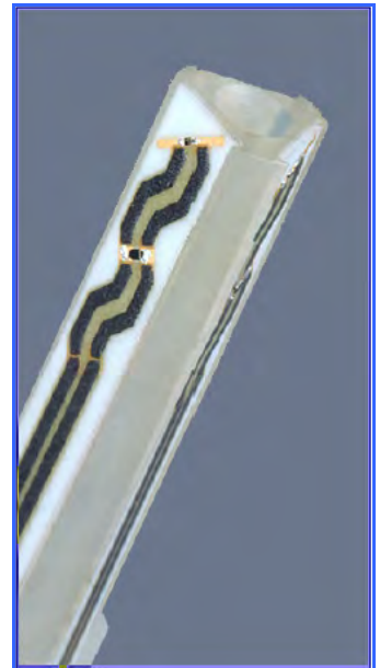
Figure 7. EX3DV3 E-field Probe
