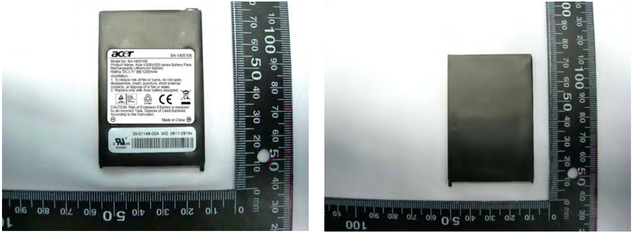
Figure 2. Lepto Battery(Li-ion 3.7V, 1250mAh )
