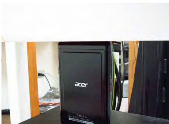
Fig.4 EUT Primary Portrait mode to flat phantom
