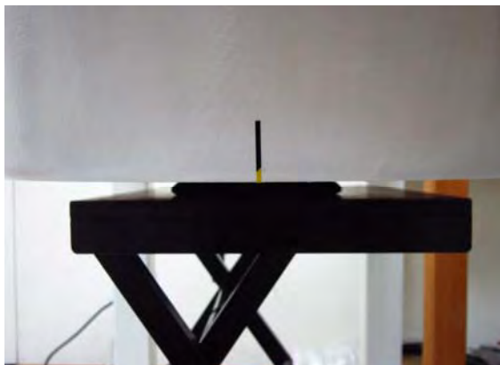
Fig.3 EUT Lap held mode to flat phantom
