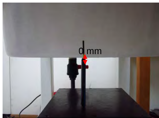
Fig.5 EUT Primary Landscape mode to flat phantom
