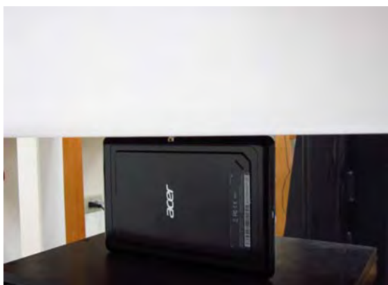
Fig.5 EUT Primary Landscape mode to flat phantom
