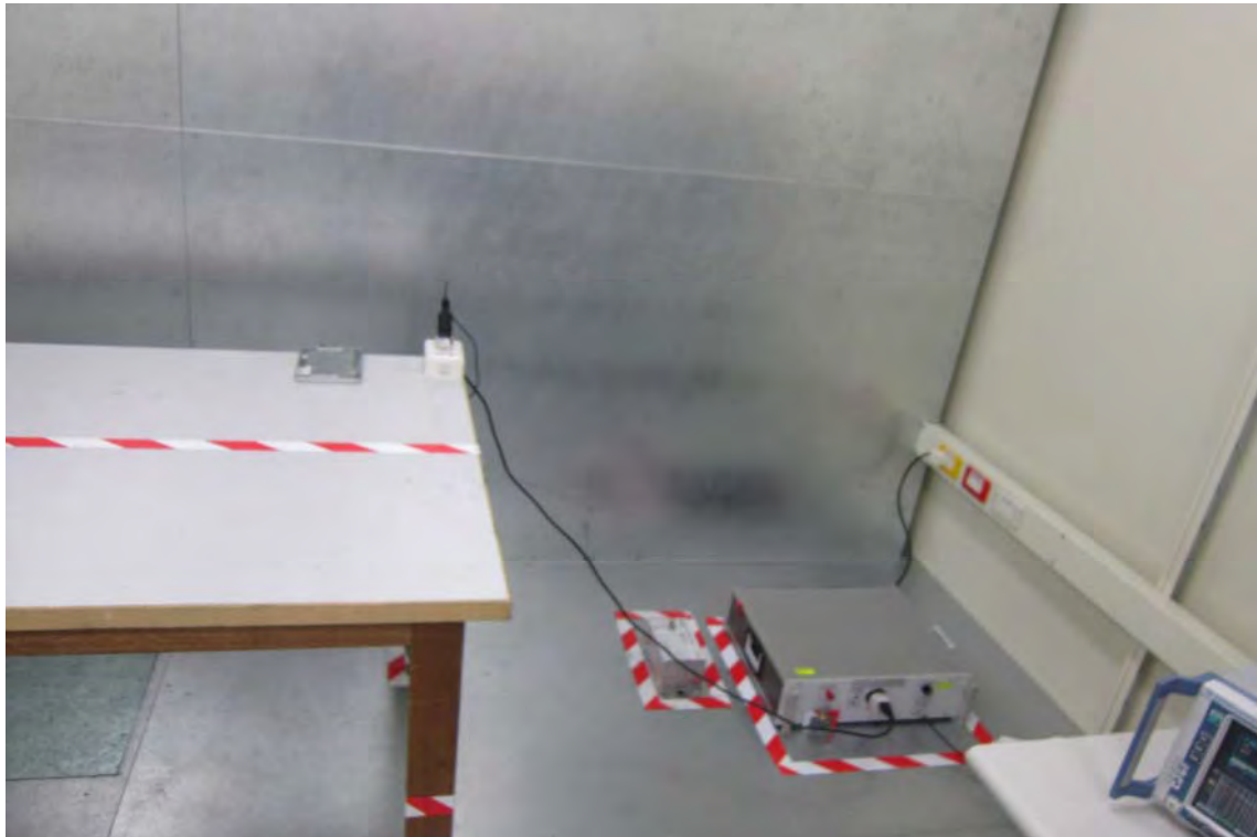
Conducted Emission Set up Photo (DELTA)
