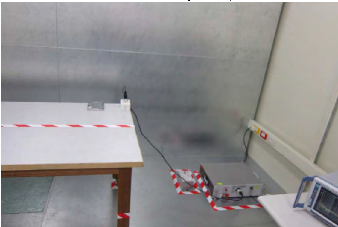
Conducted Emission Set up Photo (LITEON)
