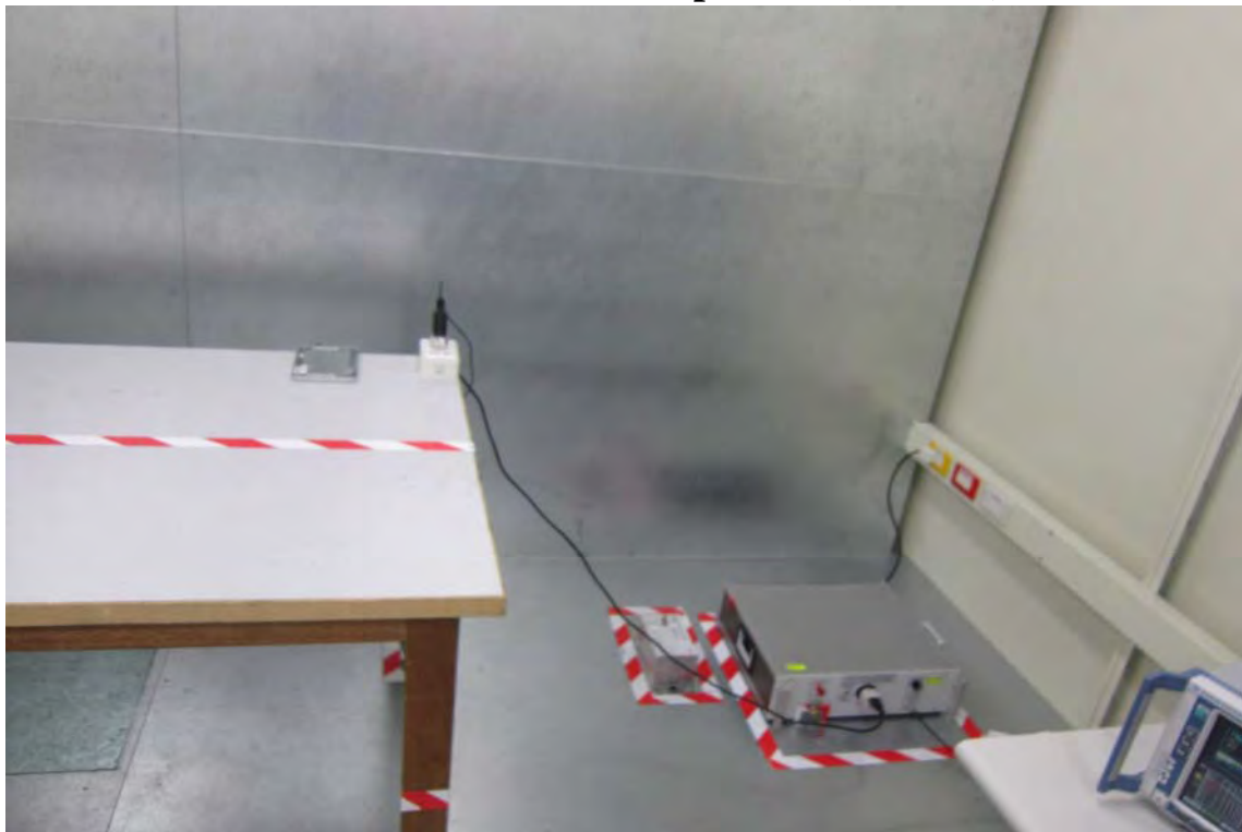
Conducted Emission Set up Photo (DELTA)
