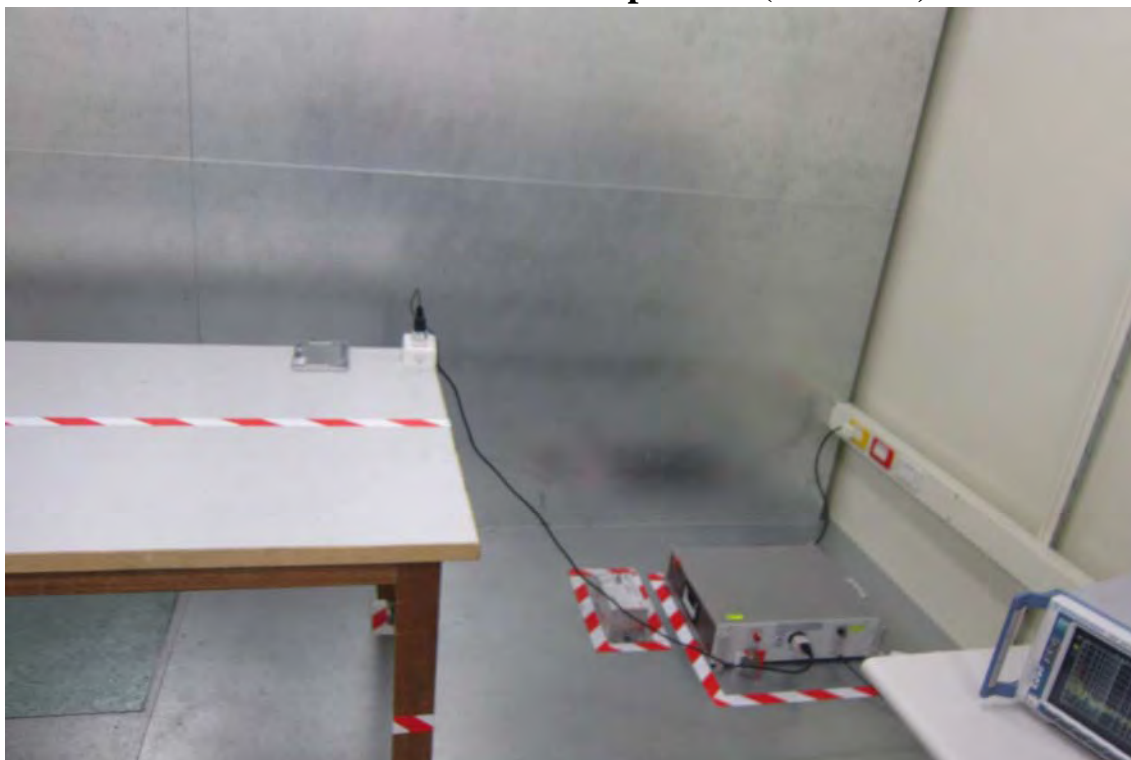
Conducted Emission Set up Photo (LITEON)
