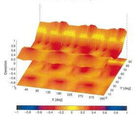
Probe isotropy for  $E_{01}$ : probe rotated  $\phi=0^\circ$  to 360°, tilted from field propagation direction  $\vec{k}$  Parallel to the field propagation ( $\psi=0^\circ-90^\circ$ ) at 30 GHz: deviation within  $\pm 0.26$  dB Parallel to the field propagation ( $\psi=0^\circ-90^\circ$ ) at 60 GHz: deviation within  $\pm 0.38$  dB
