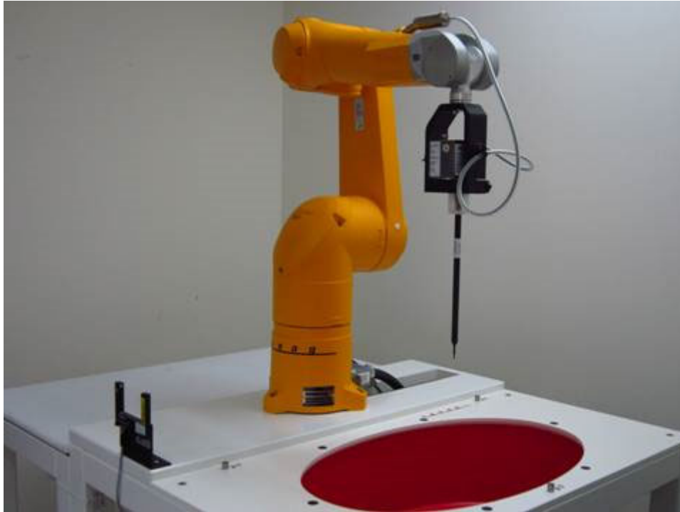
Fig.1 Photograph of the SAR measurement system
