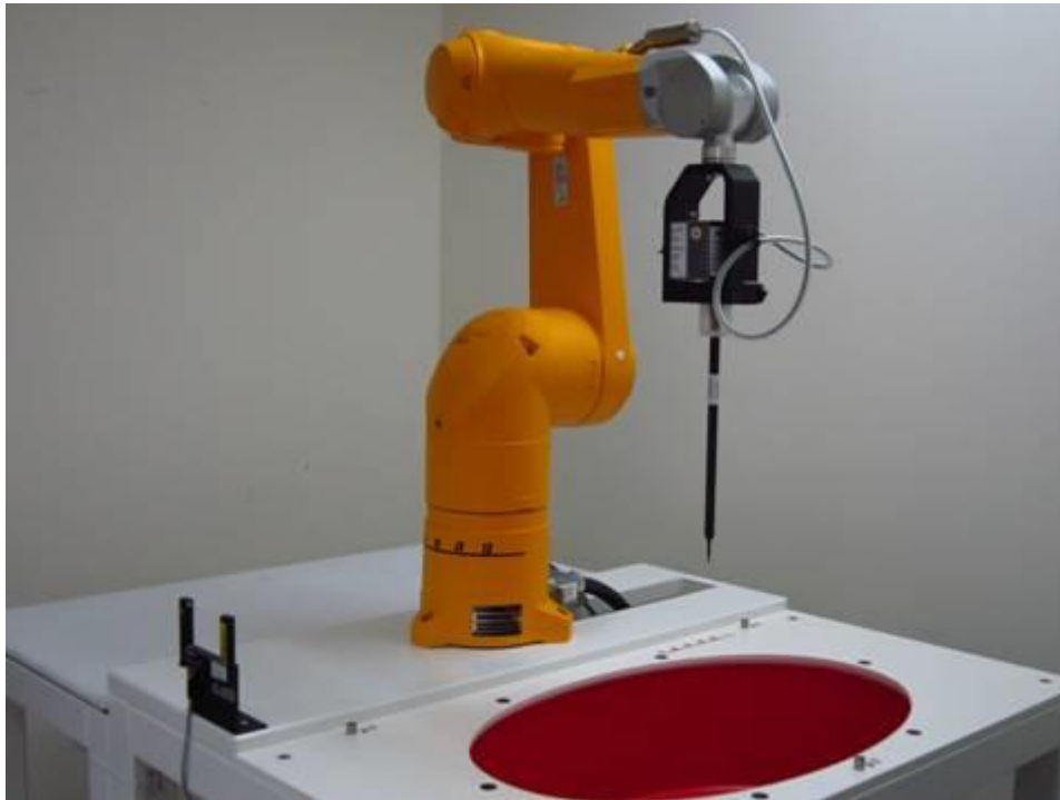
Fig.1 Photograph of the SAR measurement system
