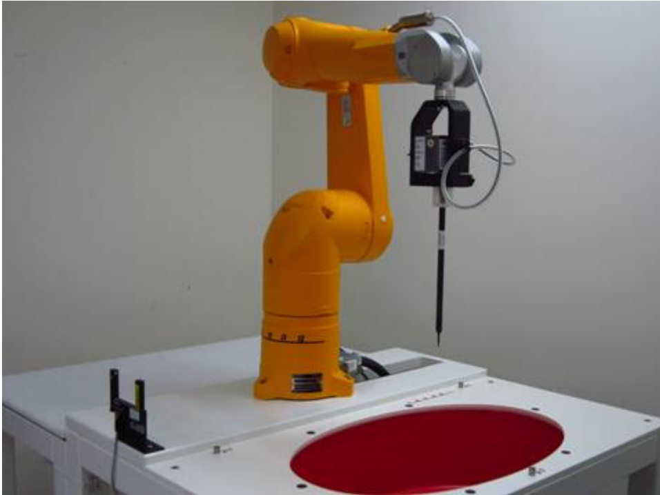
Fig.1 Photograph of the SAR measurement system
