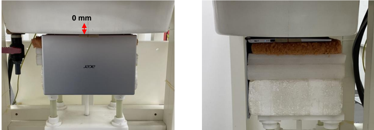
Fig.3 EUT Bottom side to flat phantom
