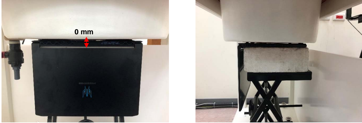
Fig.3 EUT Bottom side to flat phantom
