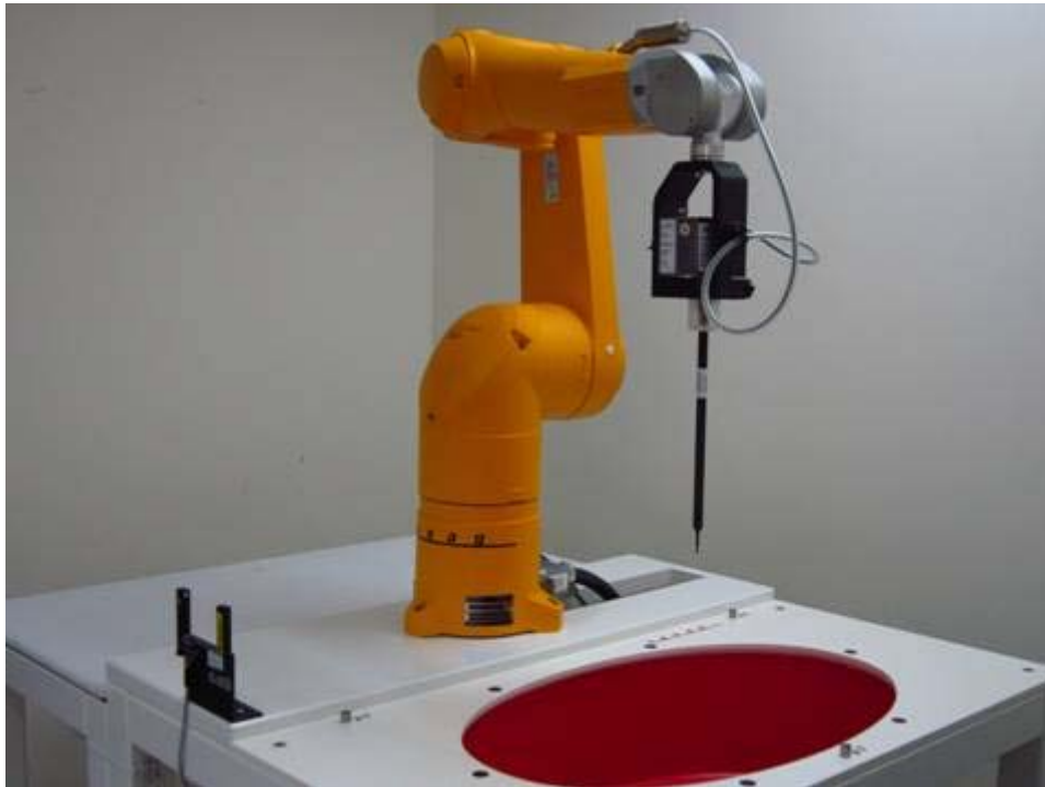
Fig.1 Photograph of the SAR measurement system
