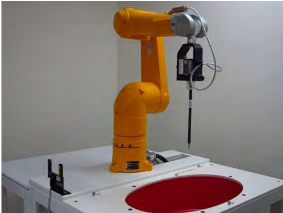
Fig.1 Photograph of the SAR measurement system
