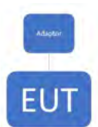
Fig. 2-2 Conducted (Antenna Port) Emission Configuration
