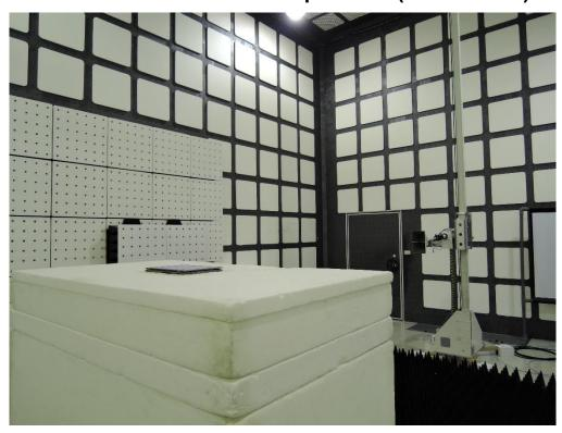
TB Radiated Emission Set up Photos (Front View)
