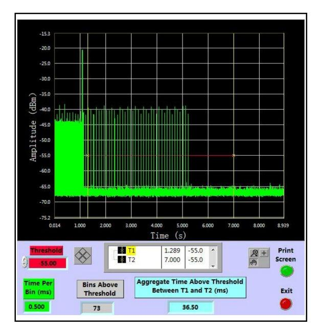
NOTE: Result time begin at T1 which was 60MS behind the radar signal trigger time.
