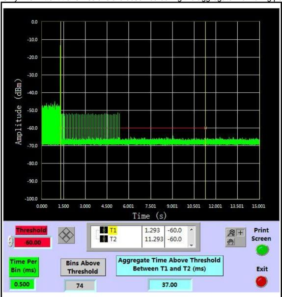
NOTE: Type 0 Radar signal trigger at T1, channel stop data transmission and move.
