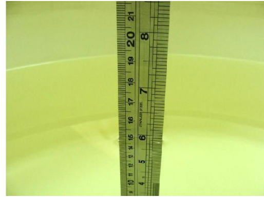
Fig 5.2 Photo of Liquid Height for Body SAR
