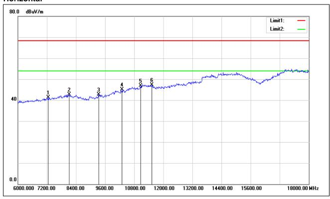
Test Mode: TX / IEEE 802.11n HT 40 MHz / 5795MHz /(CH High)
