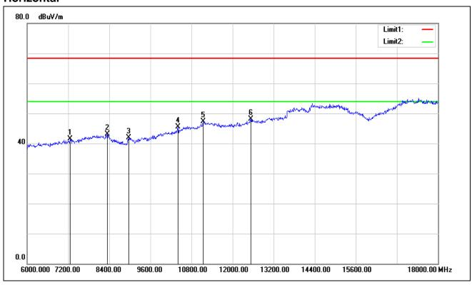
Test Mode: TX / IEEE 802.11n HT 20 MHz / 5240MHz /(CH High)
