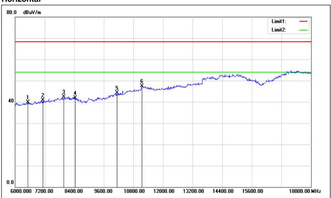
Test Mode: TX / IEEE 802.11n HT 20 MHz / 5200MHz /(CH Mid)
