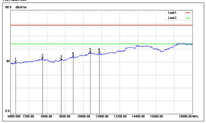
Test Mode: TX / IEEE 802.11n HT 40 MHz / 5190MHz /(CH Low)
