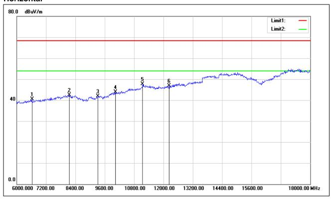
Test Mode: TX / IEEE 802.11n HT 20 MHz / 5825MHz /(CH High)
