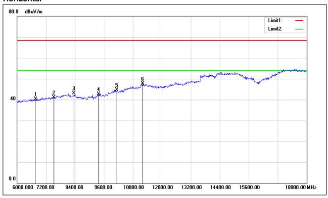
Test Mode: TX / IEEE 802.11n HT 40 MHz / 5270MHz /(CH Low)
