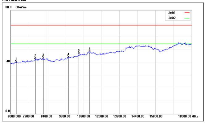
Test Mode: TX / IEEE 802.11n HT 20 MHz / 5300MHz /(CH Mid)
