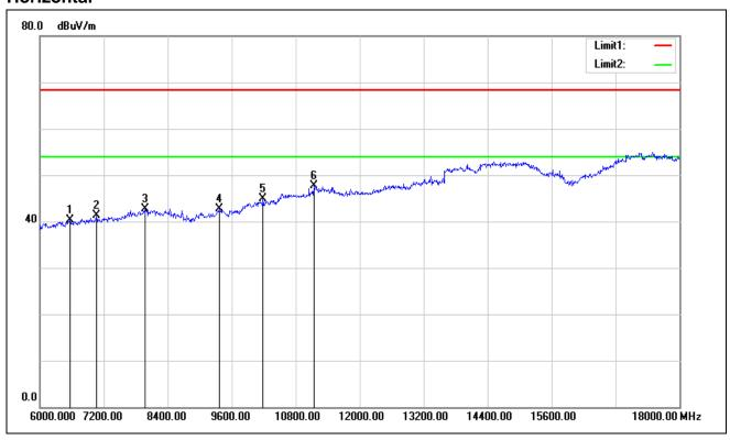
Test Mode: TX / IEEE 802.11n HT 40 MHz / 5310MHz /(CH High)
