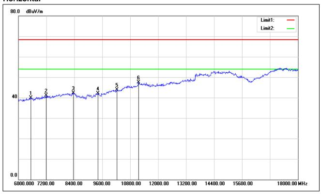
Test Mode: TX / IEEE 802.11n HT 20 MHz / 5700MHz /(CH High)
