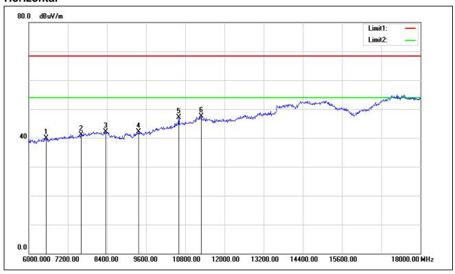
Test Mode: TX / IEEE 802.11n HT 20 MHz / 5320MHz /(CH High)
