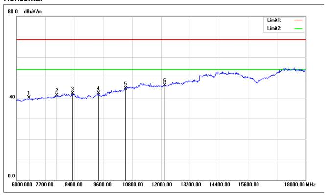
Test Mode: TX / IEEE 802.11n HT 20 MHz / 5785MHz /(CH Mid)
