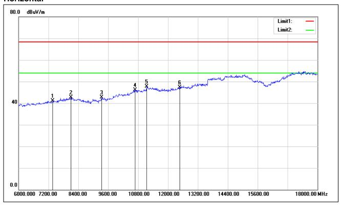
Test Mode: TX / IEEE 802.11n HT 40 MHz / 5550MHz /(CH Mid)
