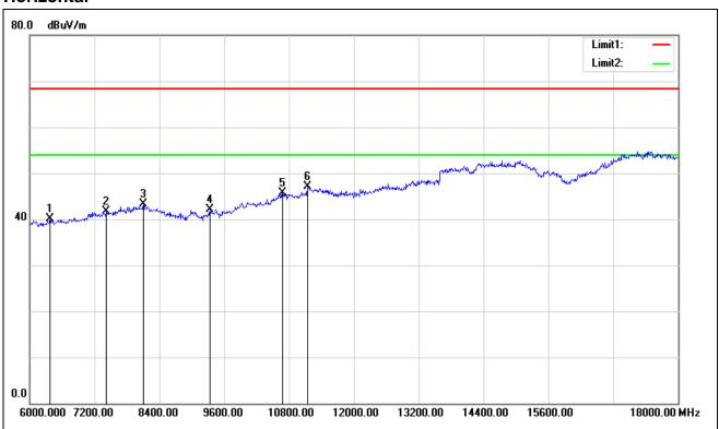
Test Mode: TX / IEEE 802.11n HT 40 MHz / 5670MHz /(CH High)
