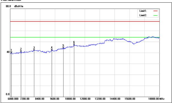
Test Mode: TX / IEEE 802.11n HT 20 MHz / 5180MHz /(CH Low)
