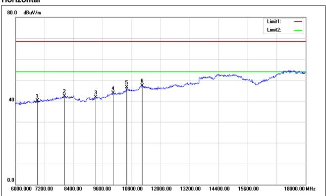
Test Mode: TX / IEEE 802.11n HT 20 MHz / 5580MHz /(CH Mid)
