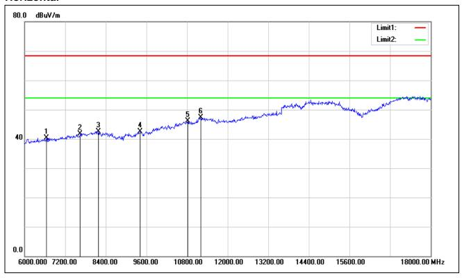
Test Mode: TX / IEEE 802.11n HT 40 MHz / 5755MHz /(CH Low)
