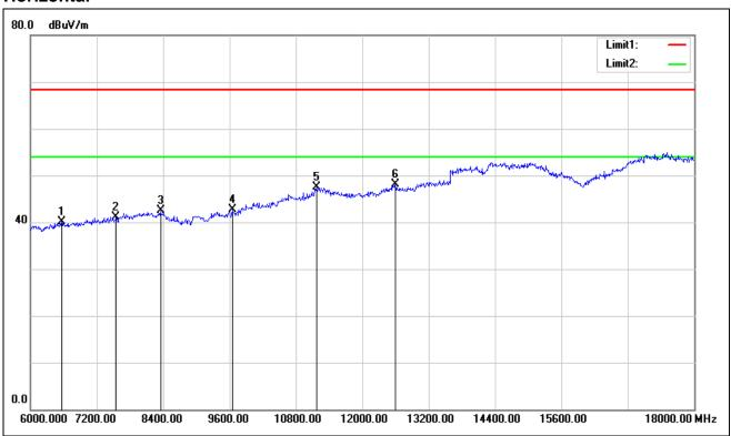
Test Mode: TX / IEEE 802.11n HT 20 MHz / 5745MHz /(CH Low)
