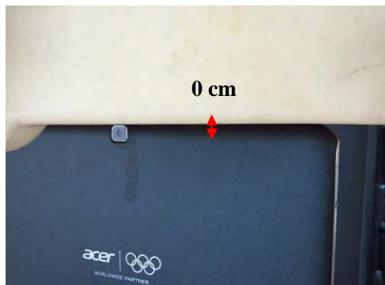
Fig.5 EUT Secondary Landscape mode to flat phantom
