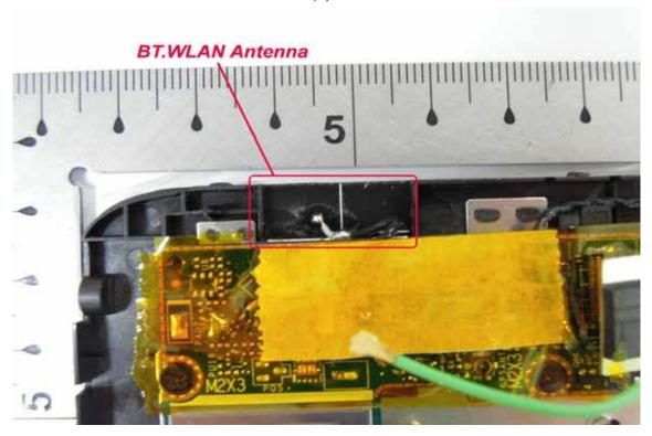
WLAN.BT Antenna (2) Inpaq PIFA Antenna
