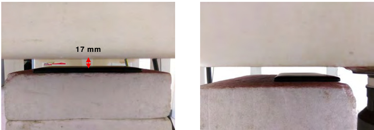
Fig.4 EUT Back side (17mm) to flat phantom
