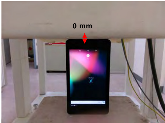
Fig.10 EUT Bottom side to flat phantom
