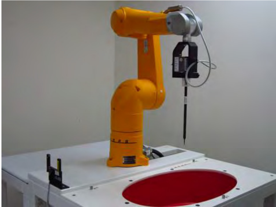
Fig.1 Photograph of the SAR measurement system
