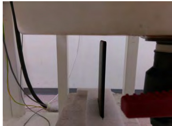
Fig.7 EUT Top side (13mm) to flat phantom
