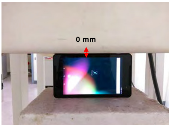
Fig.8 EUT Left side to flat phantom
