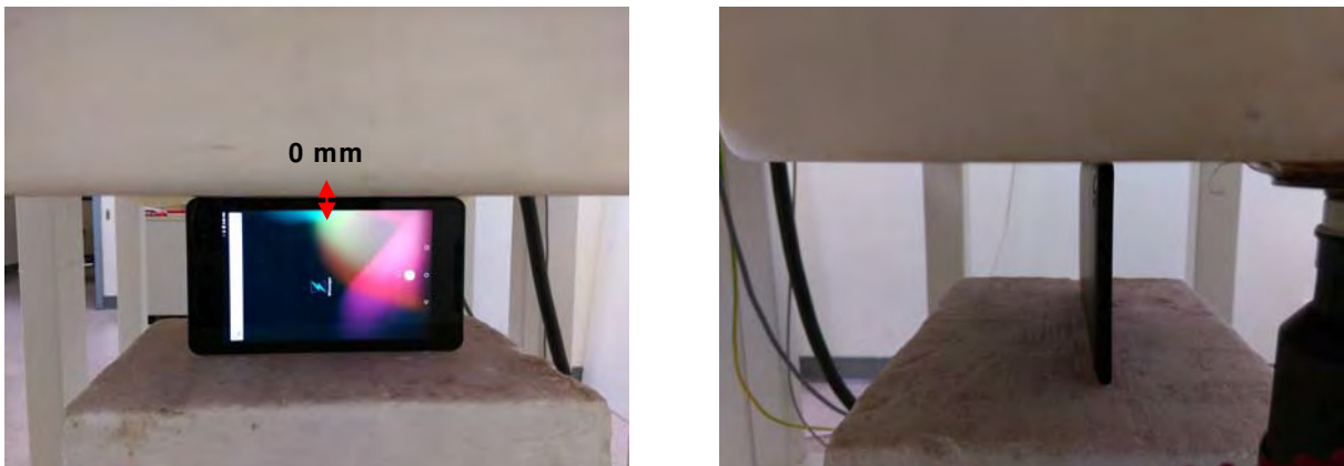
Fig.5 EUT Right side to flat phantom
