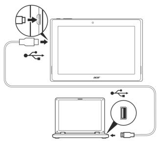
3. Swipe down from the top of the screen to display the notification area and tap **Connected as a media device** to choose whether to connect as a *Media device* (*MTP*) (the default option) or *Camera* (*PTP*).
