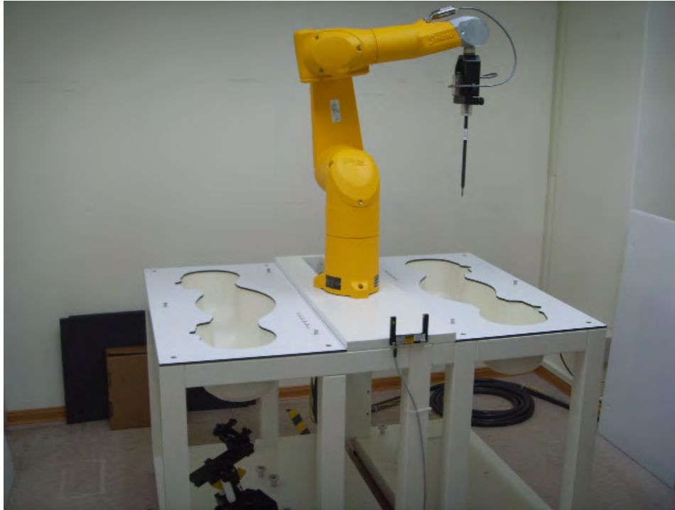
Fig.1 Photograph of the SAR measurement system
