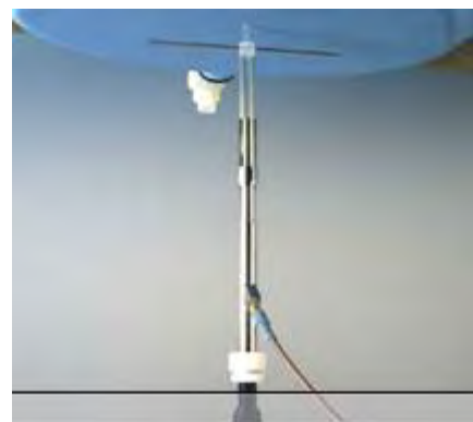
Photograph of the dipole Antenna
