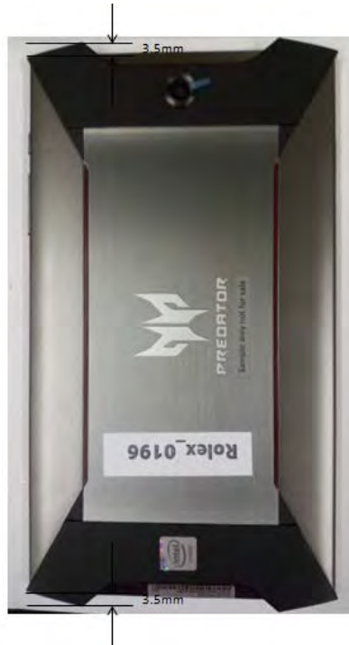
Fig.7 Antenna position of EUT (Back view)
