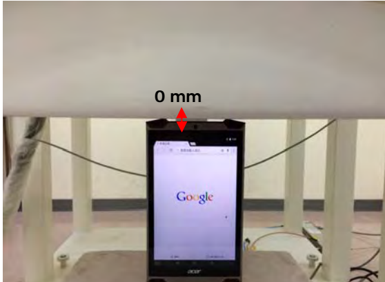
Fig.3 EUT Top side to flat phantom
