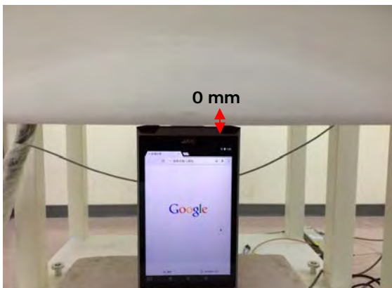
Fig.4 EUT Bottom side to flat phantom
